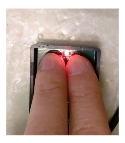
Step 2: As shown below place the wireless remote next to the programmable harness and PRESS AND HOLD the A Button. Now PRESS AND HOLD Button 1. – Continue to hold both for 5 seconds (if done properly during this time the light located in between buttons 1 and 2 will continue to flash).
