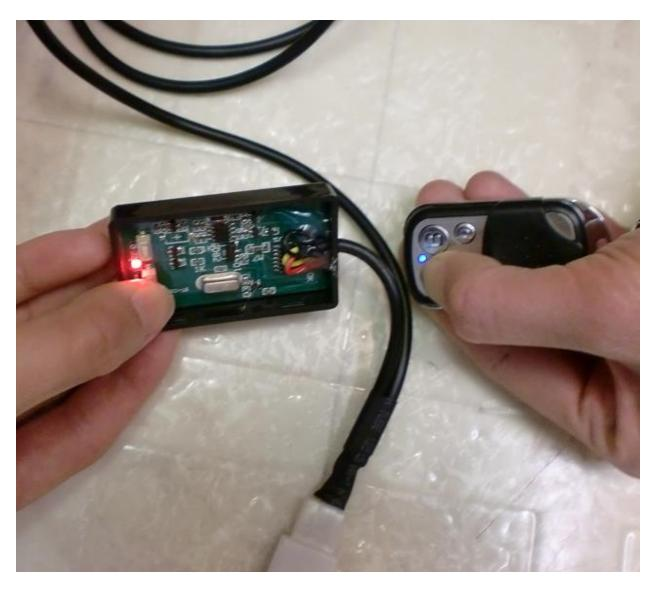
Step 3: As shown below place the wireless remote next to the programmable harness and PRESS AND HOLD the D Button. Now PRESS AND HOLD Button 2. – Continue to hold both for 5 seconds (if done properly during this time the light located in between buttons 1 and 2 will continue to flash).
