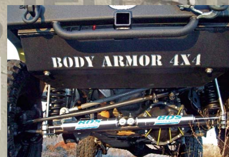
JK-5123 Front Skid Plate 3/16" steel plate includes an exclusive kickdown plate to protect electronic swaybar disconnect.
