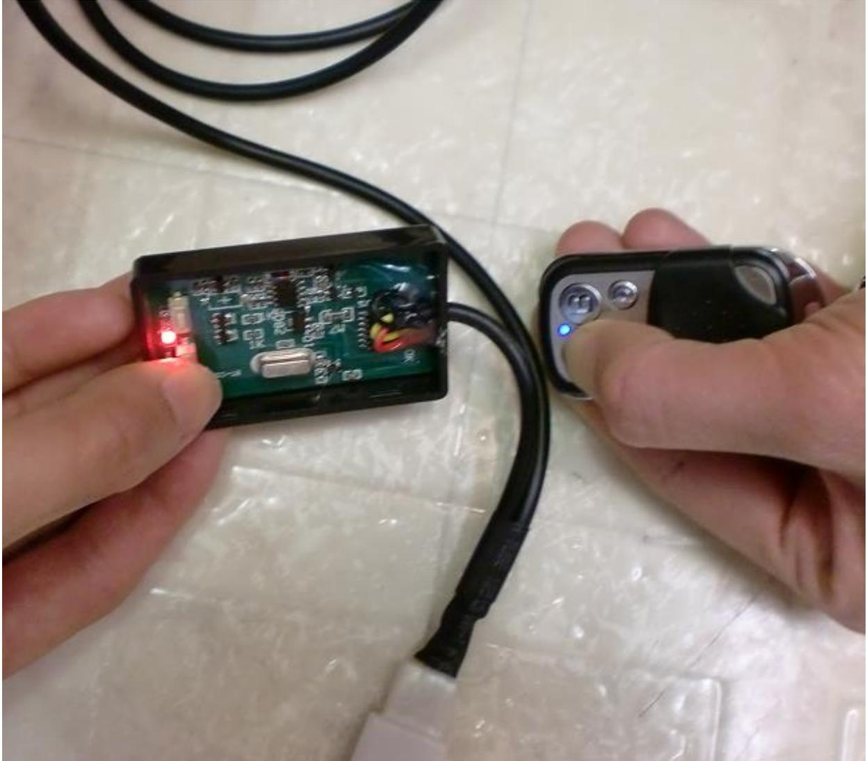
Step 3: As shown below place the wireless remote next to the programmable harness and PRESS AND HOLD the D Button. Now PRESS AND HOLD Button 2. – Continue to hold both for 5 seconds ( if done properly during this time the light located in between buttons 1 and 2 will continue to flash).
