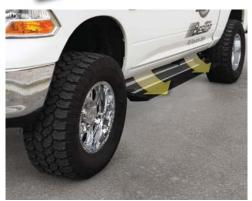
Bestop's powered running board extends down automatically when the door opens and retracts instantly when closed
