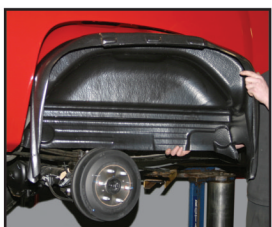
Put liner in well
